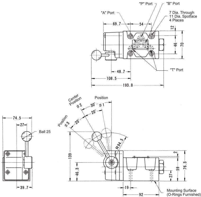
Note: For dimensions of mounting surface, please refer to the dimensional drawing of the sharable sub-plate (page 91).
