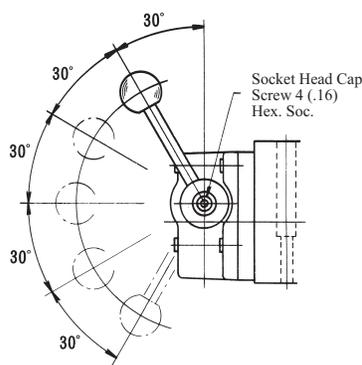
\* Handle Lever Max. Torque 30 N•m (3.06 kgf•m)
